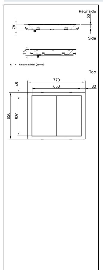
Drop-In Drop-in tempered glass top (2 GN container capacity)
